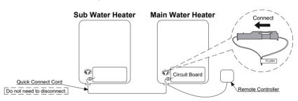
2. Then the code "CCC" or "FCC" is displayed on the Remote Controller.
